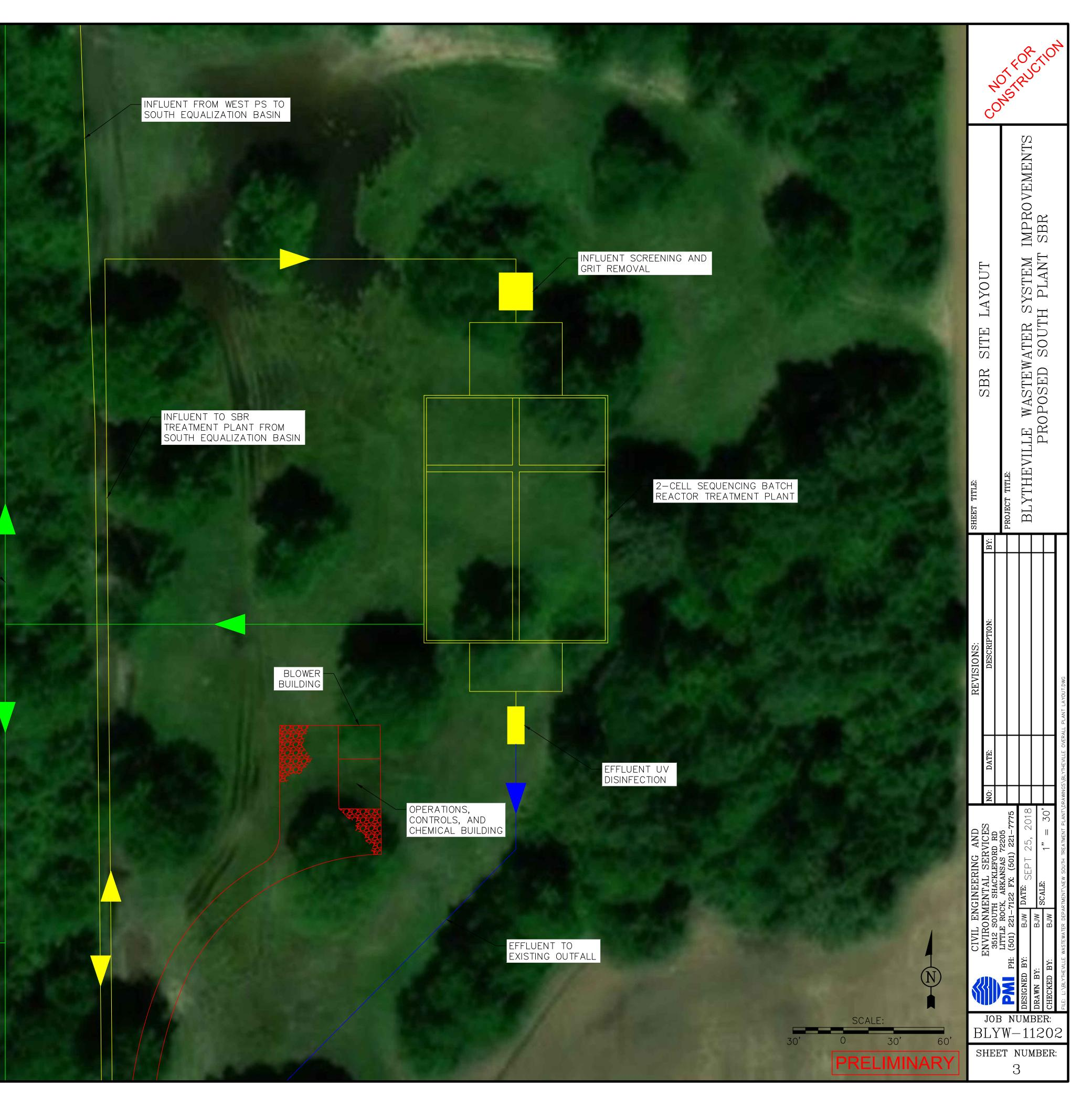
REMOVE EXISTING GRIT AND SLUDGE FROM EXISTING BIOLAC BASINS AND CONVERT TO EQUALIZATION BASINS
